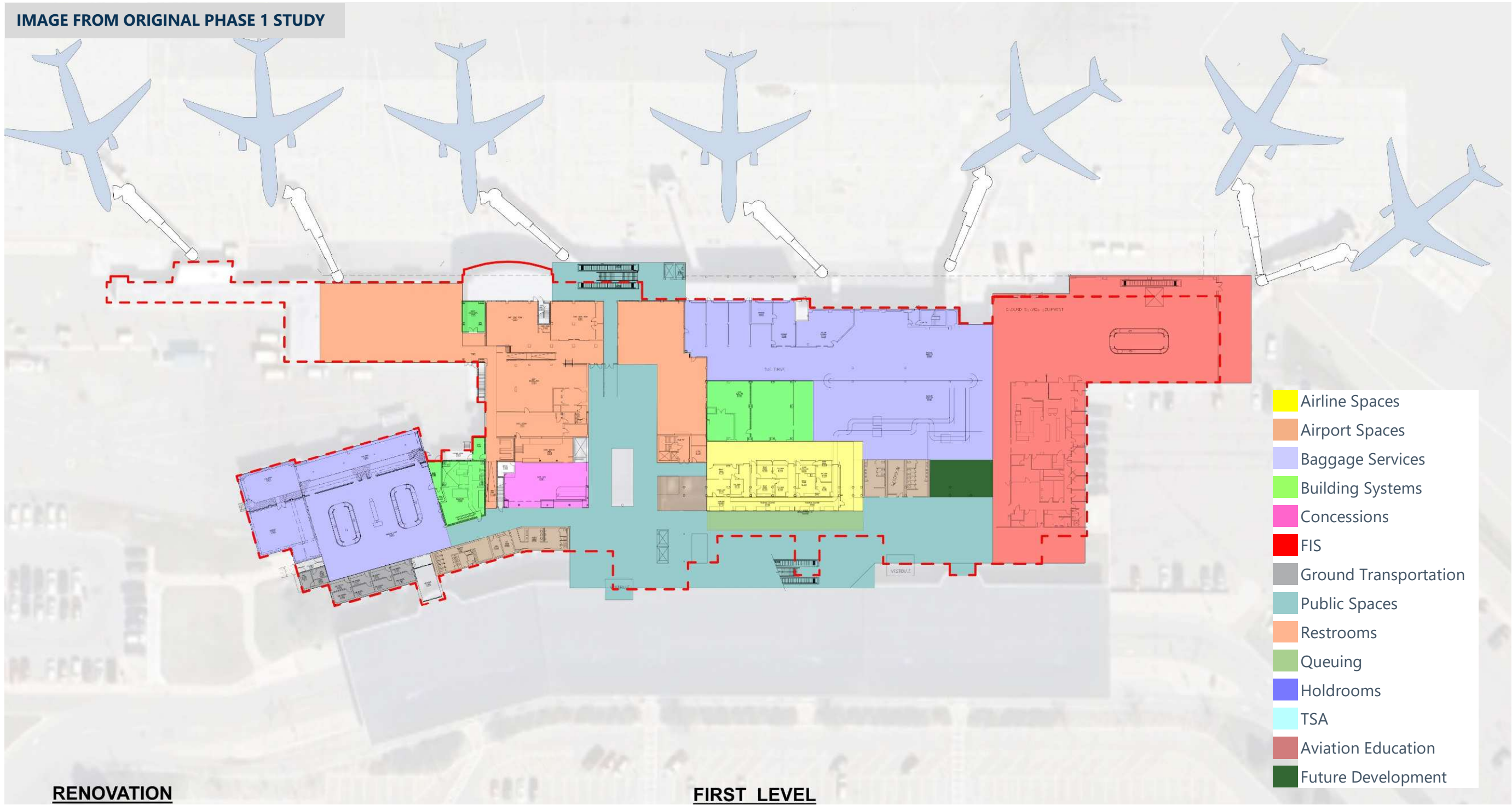
Figure 6 Original Preferred Renovation Concept – Level One
