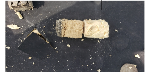
Roof T Core = Reinforced EPDM, 2 layers ISO total 3.5" on metal deck.
